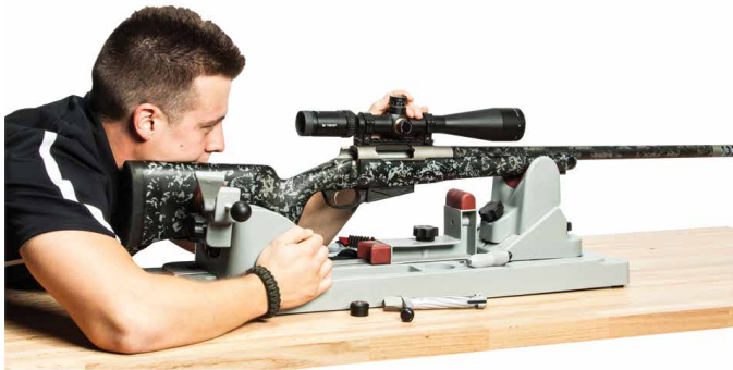
Visually bore sighting
